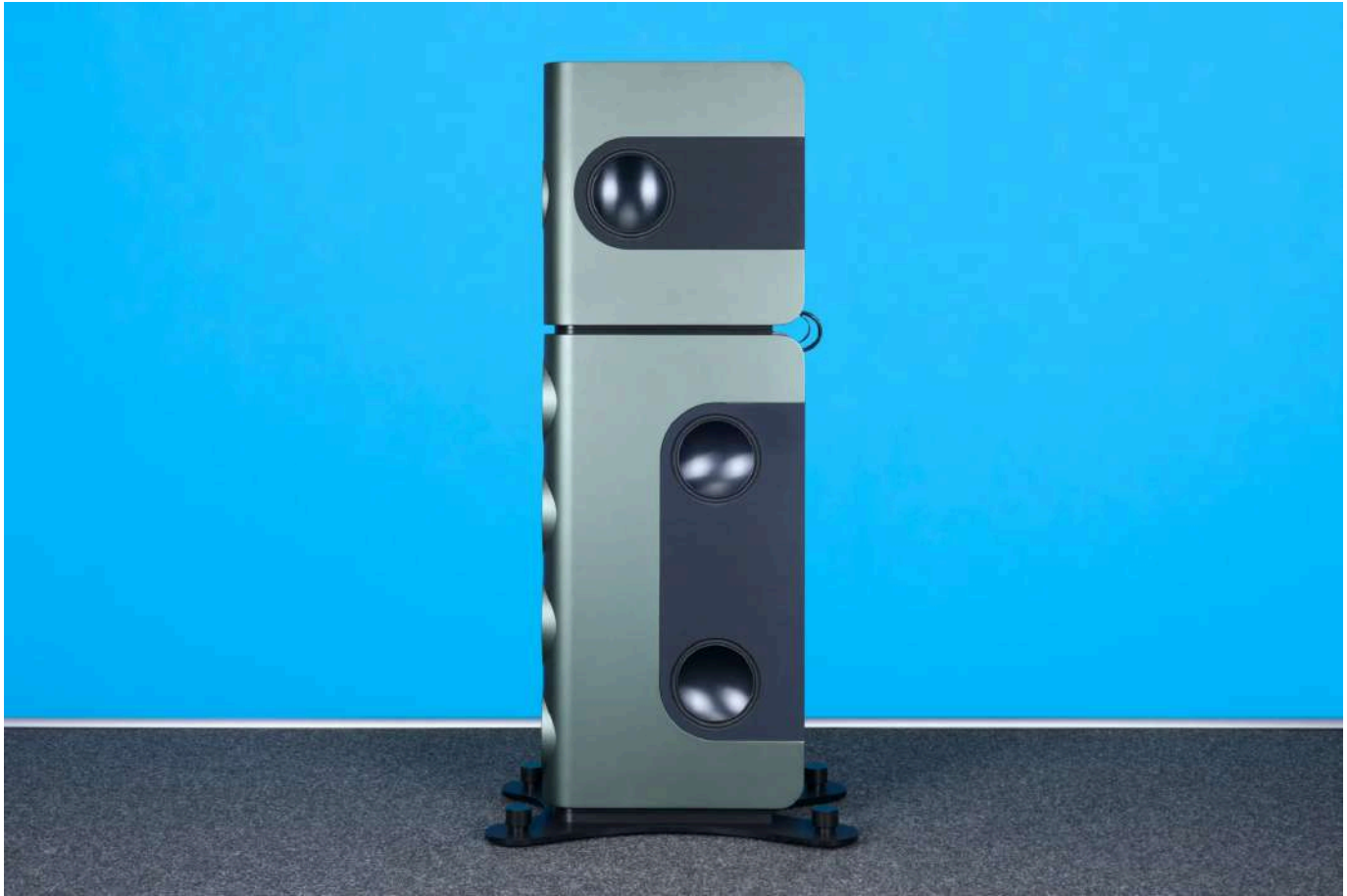
The Kii Three BXT also has bass drivers on the sides – with special tasks.
