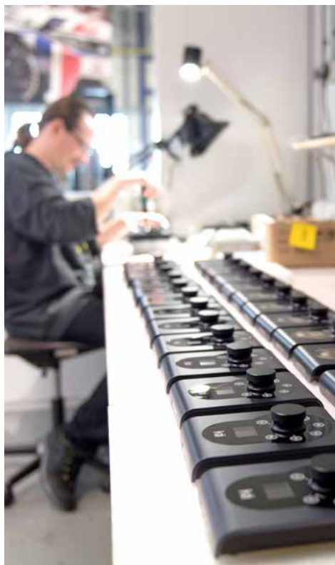
Clean room atmosphere: The solid empty housings are gradually filled with electronics and chassis before the striking aluminum inlays are added. Even the CONTROL remotes are assembled in-house by Kii Audio.
