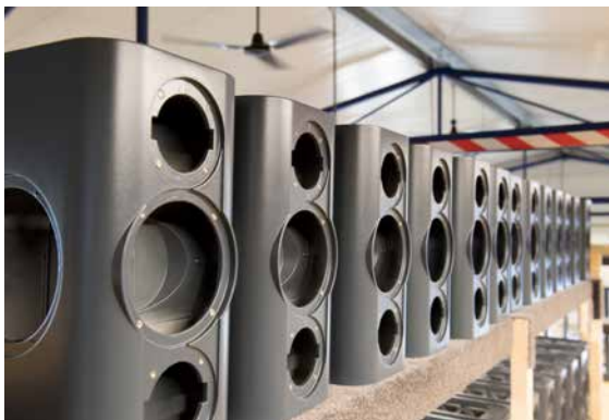
Clean room atmosphere: The solid empty housings are gradually filled with electronics and chassis before the striking aluminum inlays are added. Even the CONTROL remotes are assembled in-house by Kii Audio.
