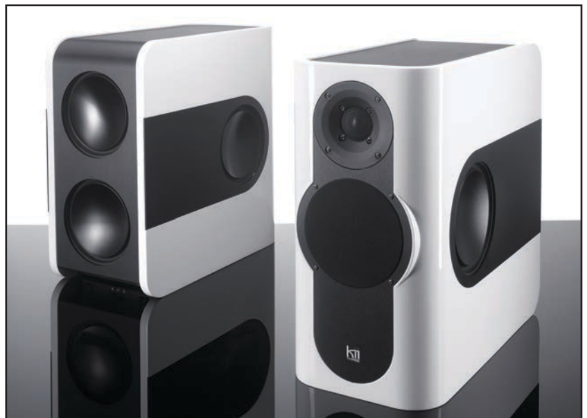
Photo 3: The Kii Three is a six-way design, with the front, the side, and the rear working together to throw the sound in one direction only without relying on a baffle. A tweeter with integrated diffraction waveguide and a 4" mid-driver hidden by a black cloth grill in the front, with four woofers with a convex aluminum surface set in an inverted surround.
