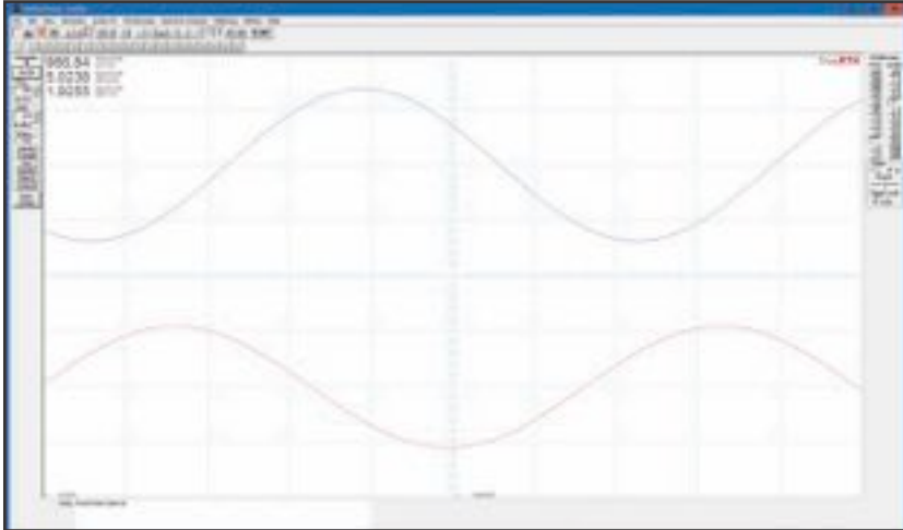
Figure 4: DSP-controlled variable phase shift between rear- and side-firing woofers controls directivity to below 100 Hz.
